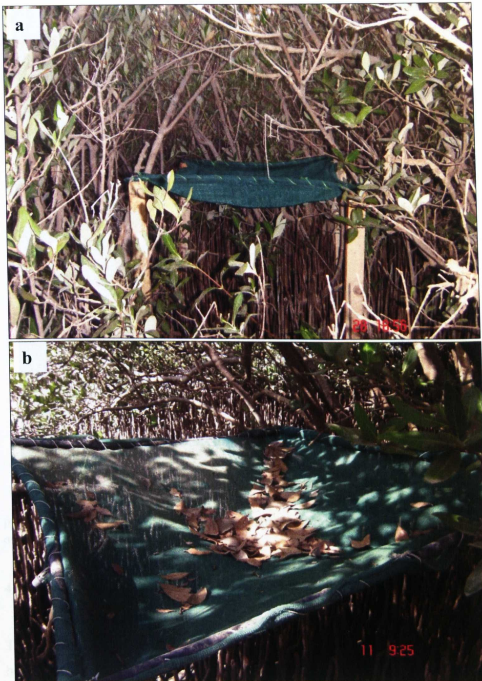
Plate 4.1 (a,b) A 1 m 2 litter trap suspended under mangrove trees on the Red Sea coast, Saudi Arabia.
