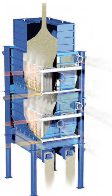
FIG. 3. Plate bank heat exchangers (dryers) are energy efficient and can offer greater operational flexibility.
