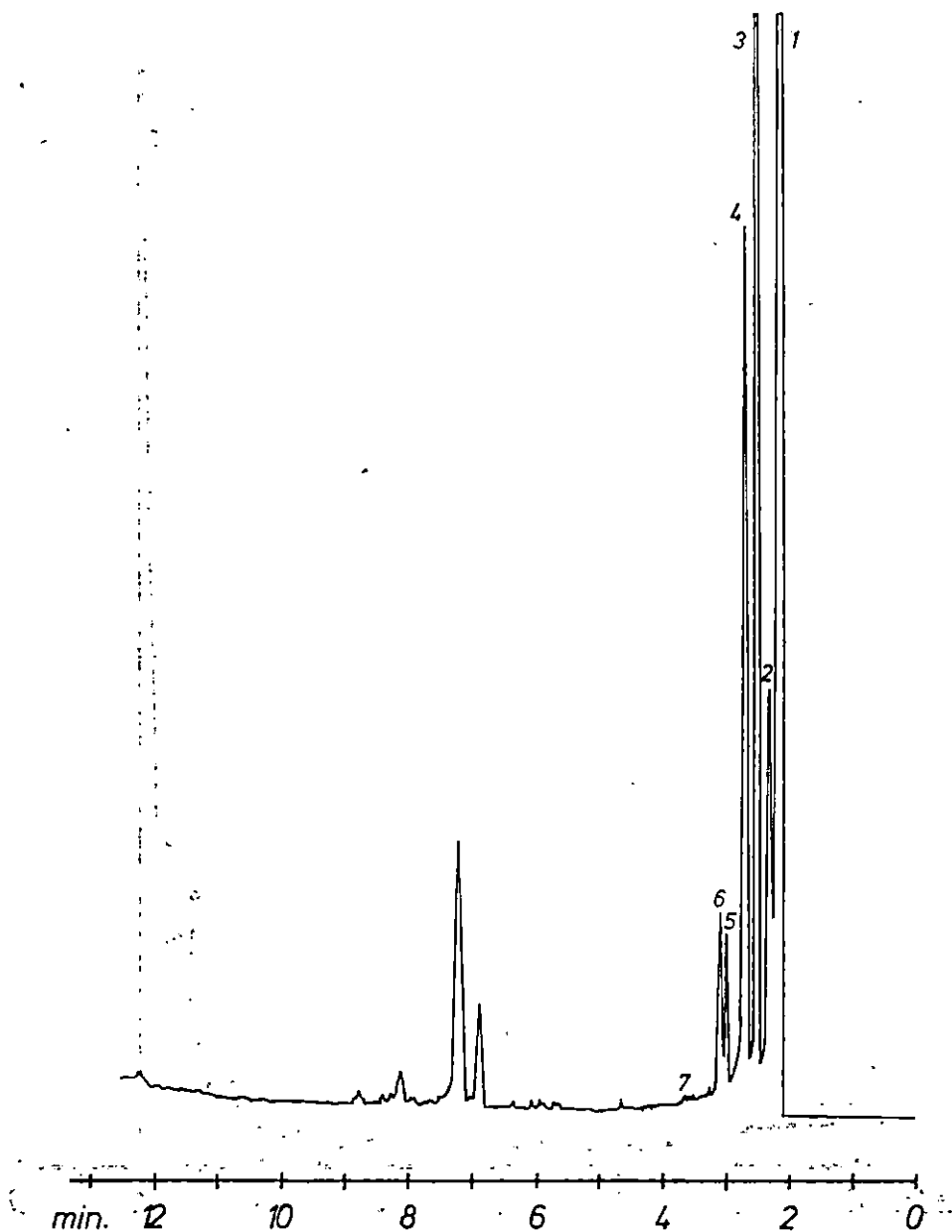
Sl. — Fig. 14. Kromatogram terpentinskog ulja Zadar 4 — Chromatogram of turpentine of the sample Zadar 4: 1 = \alpha -pinen — \alpha -Pinene, 2 = kamfen — Camphene, 3 = \beta -pinen — \beta -Pinene; 4 = \Delta^3 -karen — \Delta^3 -Carene, 5 = limonen — Limonene, 6 = \gamma -terpinen — \gamma -Terpinene, 7 = terpinolen — Terpinolene
